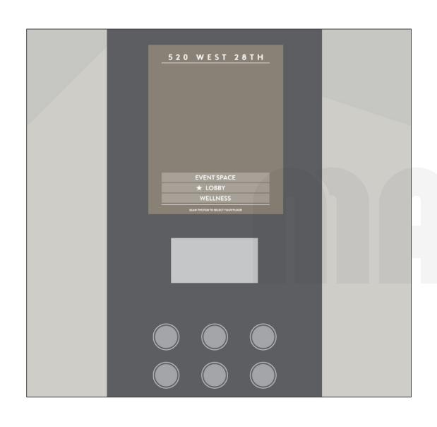
The touchscreen display shows the open accessible floors as unlit buttons which can be selected.
