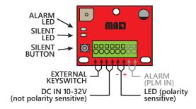
To change the volume of the alarm sound, hold the button (or keyswitch) continuously until the alarm is at the desired volume, then release.
