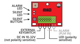
The ALARM (PLM IN) terminals are optional; they are typically not used when connecting to a RATH® SmartPhone. When the ALARM (PLM IN) contacts are open, the board will work as described above. When they are closed, the alarm sound and ALARM LED will remain off, and the SILENT LED will flash once every 4 seconds.
