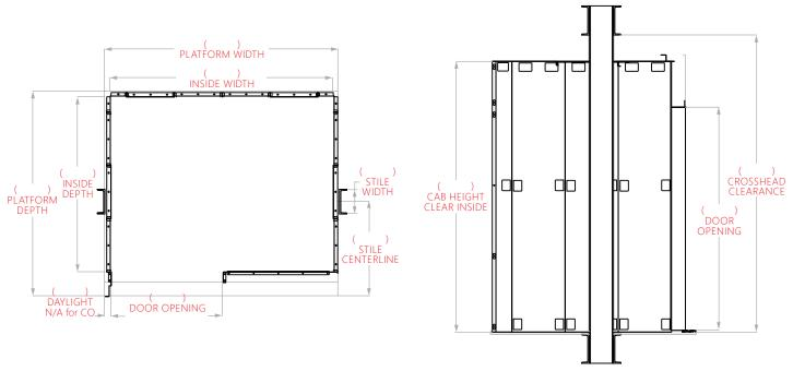
NOTE: Interior dimensions are conventionally  $2^{\circ}$  offset from the edge of the platform. If no interior dimensions are specified then the maximum possible will be provided. If interior dimensions are specified then they will be accommodated so long as it would not exceed the platform dimensions. Please confirm return widths for center opening cars otherwise they will be assumed to be equal.
