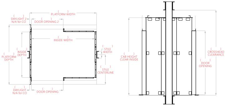
NOTE: Interior dimensions are conventionally 2" offset from the edge of the platform. If no interior dimensions are specified then the maximum possible will be provided. If interior dimensions are specified then they will be accommodated so long as it would not exceed the platform dimensions. Please confirm return widths for center opening cars otherwise they will be assumed to be equal.
