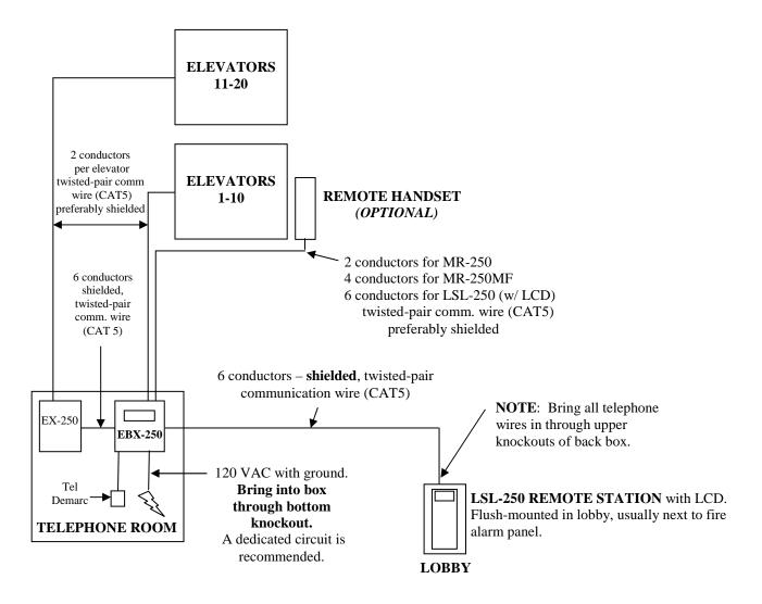
NOTE: This wiring diagram supersedes the wiring diagram provided with the LS-250 Rescue Station.
